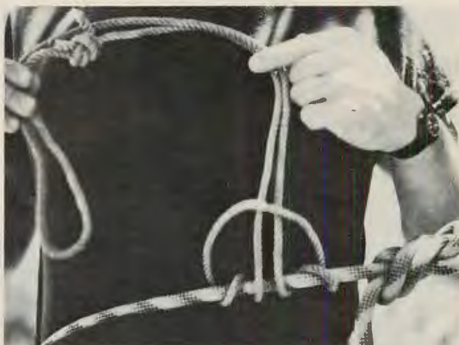
Prusik-Knot System. Step 3: Repeat previous step. Pulled tight, prusik knot "grabs" climbing rope.
